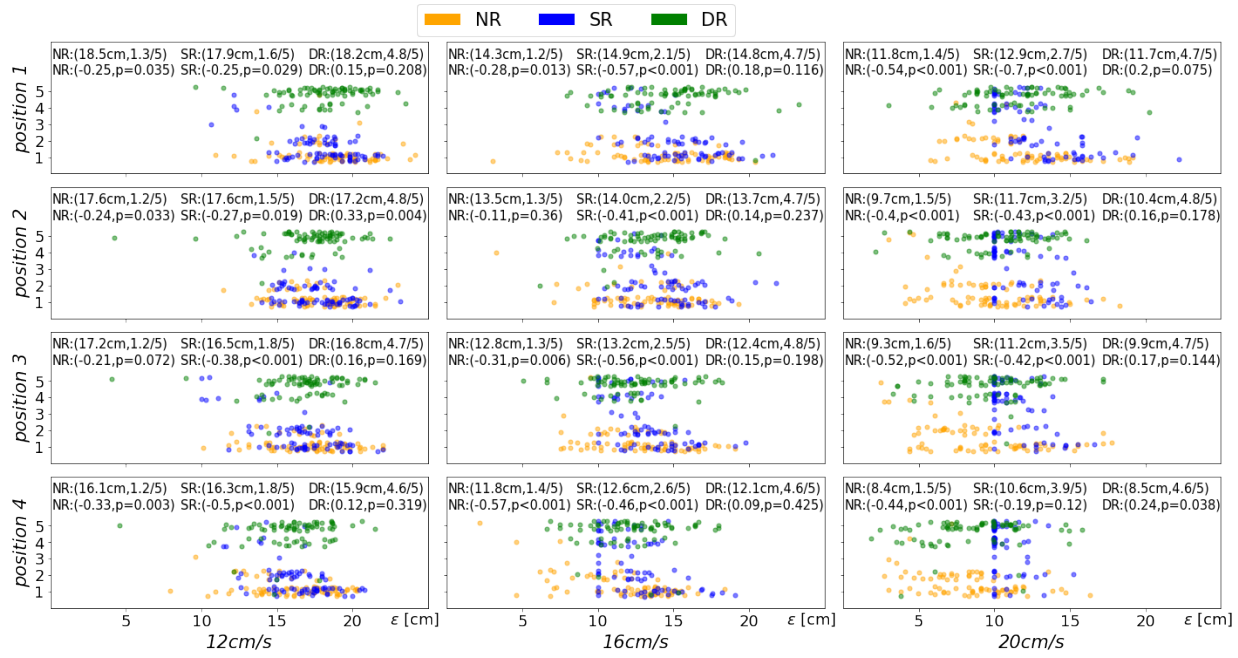
Fig. 5: Subjective rating of visual and haptic feedback synchronization, for each position (rows) and each ETHD speed (columns). Each scatter-plot panel has the gap \epsilon between the virtual and physical disks on the x axis, and the rating on a five-point Likert scale as the y axis. Each panel shows the dots for the 25 participants, three repetitions, and three conditions, with cumulative transparency. At the top of each panel, the first row gives the average \epsilon and average rating, for each condition; the second row gives Spearman's rank correlation between rating and \epsilon .
