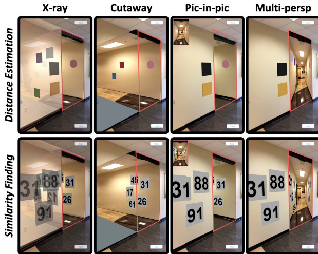
Figure 2: Disocclusion with four AR interfaces (columns) in two additional tasks (rows). For one task, the user is asked to find the rectangular color patch closest to the pink disk (top row). For the second task, the user is asked to find the number that appears twice.
